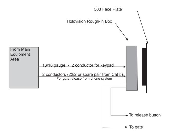
**Note on Essex Wiring:** Electric motorized gates require only a contact closure from the S12 keypad. Electric strikes or mag locks can draw several amps, and the appropriate wire size should be calculated. Longer runs will require a heavier gauge wire.
