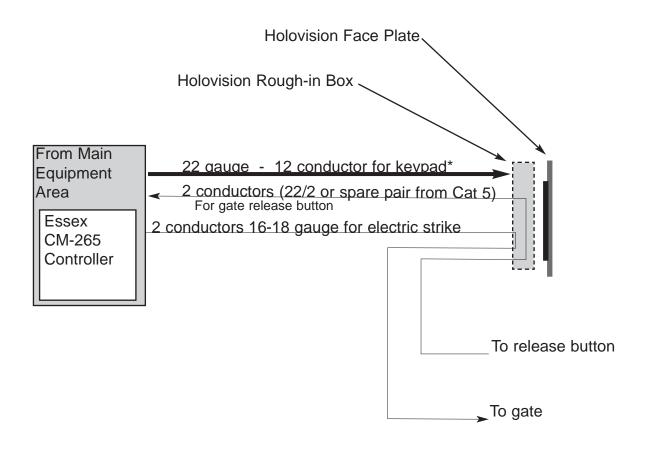
**Note on Essex Wiring:** Wires to connect to the **gate strike** and to the **gate release button** are required (see above). Electric motorized gates require only a contact closure from the CM-265. Electric strikes or mag locks can draw several amps, and the appropriate wire size should be calculated, however 16 ga should be adequate in most instances. Longer runs will require a heavier gauge wire.
