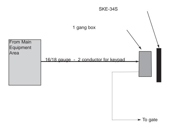
**Note on Essex Wiring:** Electric motorized gates require only a contact closure from the S12 keypad. Electric strikes or mag locks can draw several amps, and the appropriate wire size should be calculated. Longer runs will require a heavier gauge wire.
